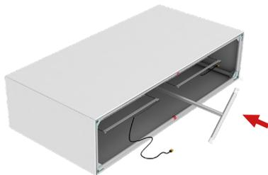
**Position** and push pole onto the red indicators at top of frame. **Lock** the bottom of the pole by firmly sliding or knocking the pole into place.
