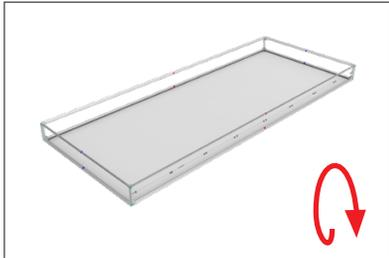
**Step 10:** Take out the LED Lights and **gently** unroll on the graphic with lights face down. **WARNING! Do not drag lights across ground or it could break the LED lights.**
