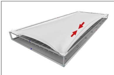
**Step 14: Turn. Position. Lock.** Insert tensioning pole into the bottom of display. Keep the pole flat until the entire pole fits inside the frame. **Turn** the pole 45°. **Position** and
