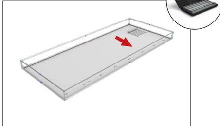
**Step 11:** Attach Light Array at top of frame onto wire harness clips.
