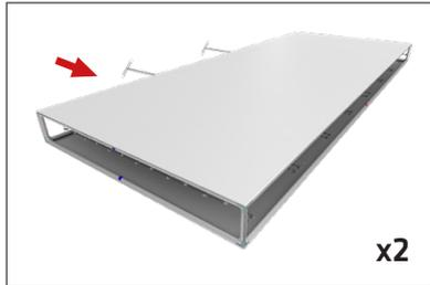
push pole onto the red indicators at top of frame. **Lock** the bottom of the pole by firmly sliding or knocking the pole into place over red indicators.
