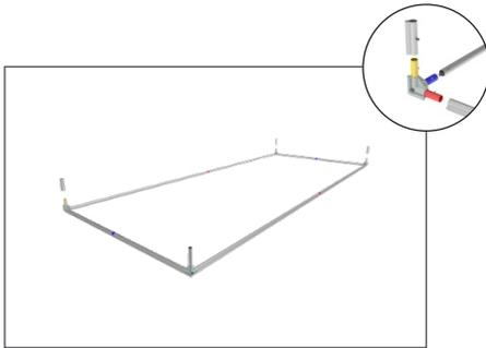
**Step 3:** Build two outer frames and connect top and bottom frames together in the corners with small connecting pipes.
