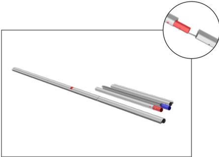
**Step 2:** Connect all corner sections to straight sections of the frame by matching color on pipes.
