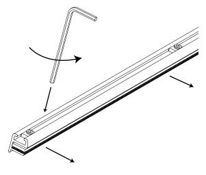
2 Attach self-adhesive graphic guides to rear of top and bottom edges of graphic
