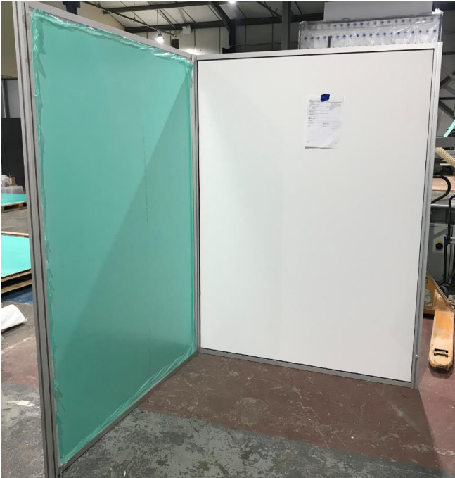
View of the front and side walls connected in a 90° angle
